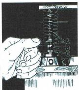
Repeat the operation for all eight valves. So far we have assumed that it will be necessary to enlarge the gap by turning the sel-screw down. This is because the gap tends to reduce with use of the engine rather than to increase. It may, however, prove necessary to reduce the gap, in which case, you will need to turn the set-screw upwards before locking.
